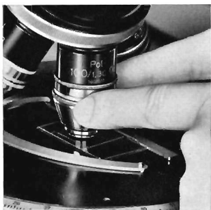
Fig. 2. Centering of the objective of the lower milled knob
