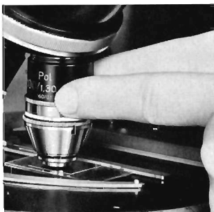
Fig. 3. Centering of the objective on the upper milled knob
