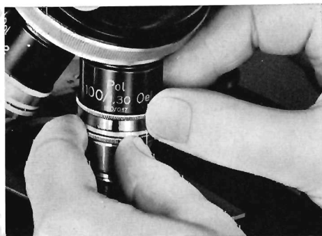
Fig. 4. Centering of the objective on both knobs simultaneously
