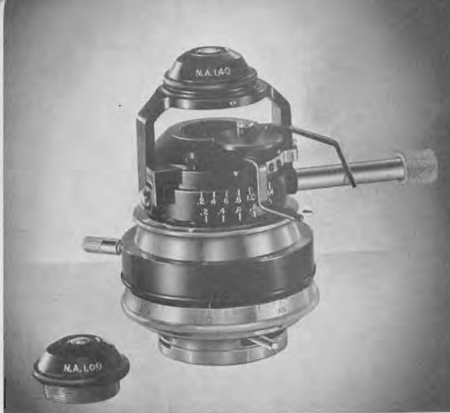
*Substage Condenser No. 532, standard equipment on No. 37.
