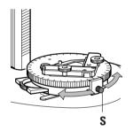
Slide in compensator red I and turn with knurled ring.
