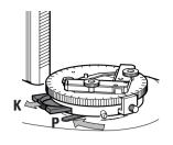
► Look into the binocular tube and move lever on analyser until the field of vision (without specimen) appears as dark as possible.
