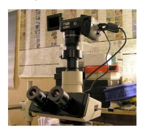
You can see how the adapters have moved the camera higher up than the CP-990, and so it is no longer parfocal with the eyepieces. Also, the view screen is kind of small, so it is trickier to get a precise focus, and the manual buttons are not as conveniently placed.
