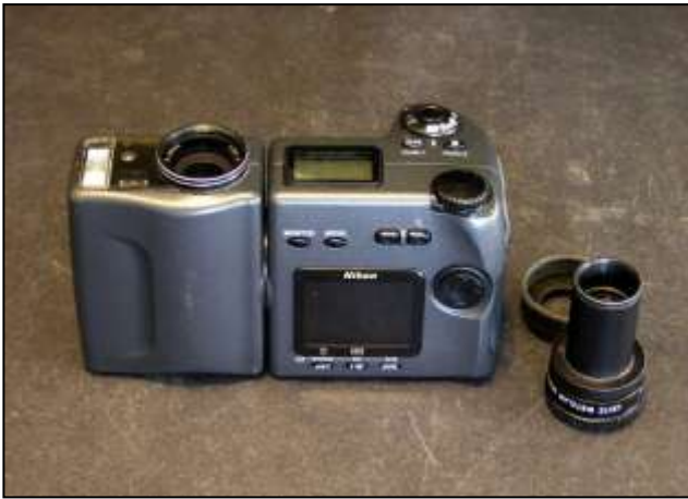
Figure 1. Nikon Coolpix 990 and Leitz Periplan 10x eyepiece, with its rubber eye guard unscrewed.
