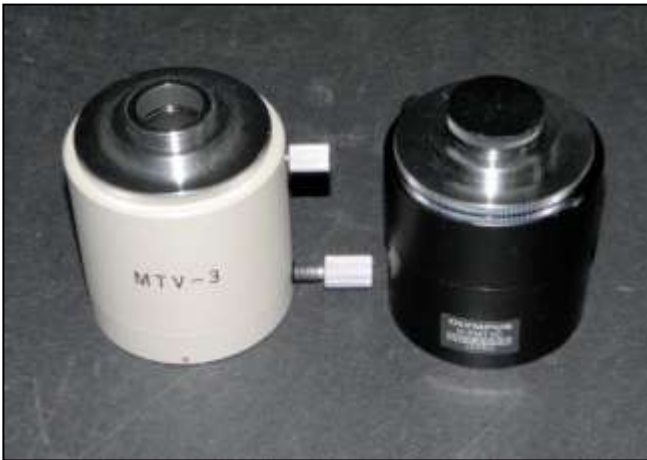
Figure 9. MTV-3 and U-PMTVC c-mount connection tubes for BH2 head flanges.
