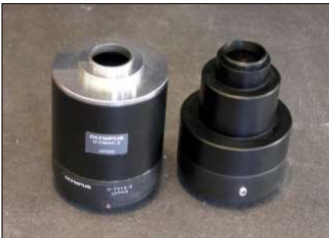
Figure 10. U-CMAD-2 (left) and U-CMAD-3 (right) c-mount connector tubes for BX heads.
