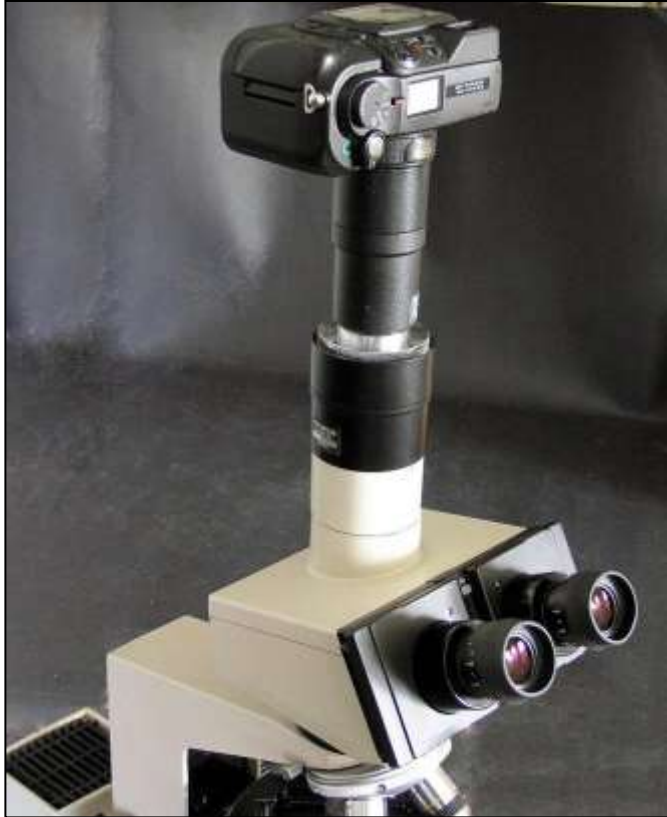
Figure 12 (right). On my BX50 microscope, a Camedia C-5050 (5 megapixels) is attached to a C3040-ADU relay adapter and U-CMAD-2 plus U-TV1x tubes.
