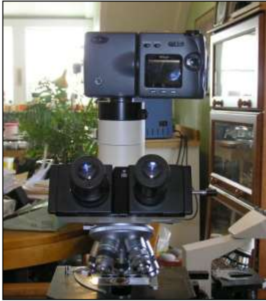
Figure 3. CP990 with a Zarf adapter, also housing a Zeiss 8x eyepiece for the relay lens.
